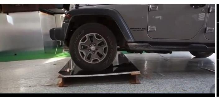
1,250 kgs pressure on H Panel aluminum reinforced composite panel
