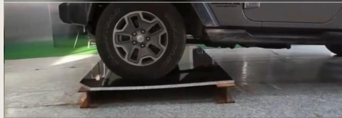
**1,250 kgs pressure on X3 - aluminum reinforced composite panel**
